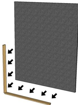
5. Apply pressure and slowly slide the panel to the proper position according to the marks. Press and roll your hands across the surface of the material to ensure you have made proper contact with the adhesive.
