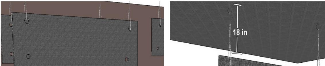
2. The grommets on the Echo Absorber Baffles are 40" apart and approximately 4" from each edge.
