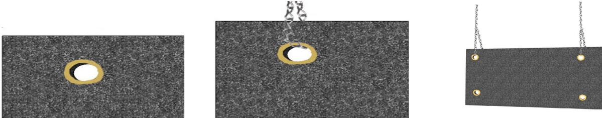
5. Cut the light duty chain into 18" sections (or whatever your desired hanging height is) and install the chain to each of the Echo Absorber Baffles.
