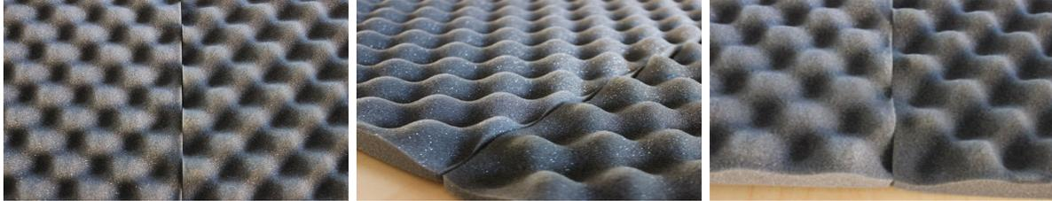
2. Measure any areas that need to be field cut on the foam and make the appropriate cuts (examples would be around beams, doorways, or if a short piece is needed).
