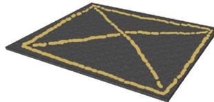
5. Line the material up with the lines you marked in Step 3 and press lightly against the material being careful not to compress the foam. Repeat step for remaining pieces of foam.
