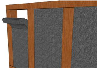
2. For overhead applications, you may need to use Insulation Supports to hold the material up inside the joist bay.
