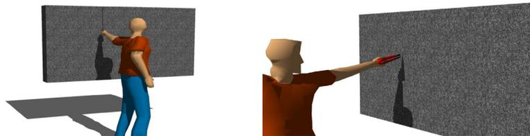
2. You can use a utility knife to cut the Quiet Batt; however, it will take multiple passes and the knife may dull quickly. If you must use a utility knife, it is sometimes helpful to compress the material along the marked line with a board or level and then cut along that compressed line.
