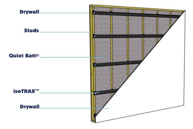
This assembly is perfect for shared walls in condominiums and apartments and a cost effective alternative to our best assembly. Use this assembly to reduce airborne and structural borne noise transfer between two rooms. This type of construction is a good solution for a variety of spaces from bedrooms to mechanical/machinery rooms.
