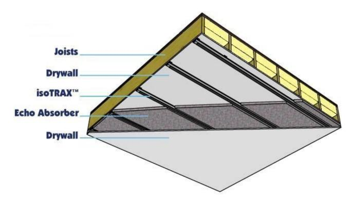
This assembly is perfect ceilings in condominiums and apartments. Use this assembly to reduce airborne and structural borne noise transfer between two rooms separated by a ceiling/floor assembly. This type of construction is a good retro fit solution for a variety of spaces from bedrooms to mechanical/machinery rooms.
