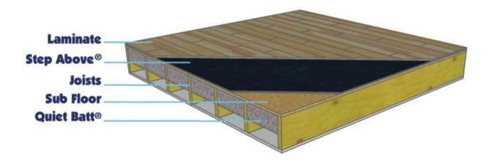
This is the best assembly for improving the soundproofing performance of Laminate floors. Use this assembly to reduce impact noise (foot fall) and airborne noise transfer between two rooms with an adjoining floor/ceiling. The Step Above<sup>®</sup> product in this assembly will also make the laminate floors sound more like hardwood. This type of construction is perfect for floors in multifamily dwellings such as condominiums and apartment buildings.
