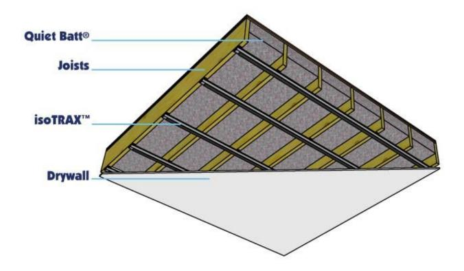
This assembly is perfect for ceilings in condominiums and apartments. Use this assembly to reduce airborne and structural borne noise transferred between two rooms separated by a ceiling/floor assembly. This type of construction is a good solution for a variety of spaces from bedrooms to mechanical/machinery rooms.
