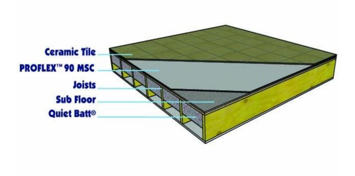
This assembly will soundproof ceramic tile and marble floors. Using this assembly will reduce impact noise (foot fall) and airborne sound transmission between adjoining rooms connected by a ceiling/floor. This type of construction is perfect for floors in multi-family dwellings such as condominiums and apartment buildings.
