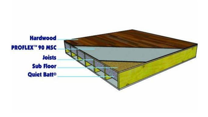
This is a great assembly to soundproof hardwood floors. Using this assembly will reduce impact noise (foot fall) and airborne sound transmission between adjoining rooms connected by a ceiling/floor. This type of construction is perfect for floors in multi-family dwellings such as condominiums and apartment buildings.
